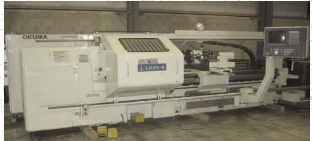
CNC LATHE OKUMA LH35N = 1 MACHINE Machining Cap \varnothing 300 X 3000
