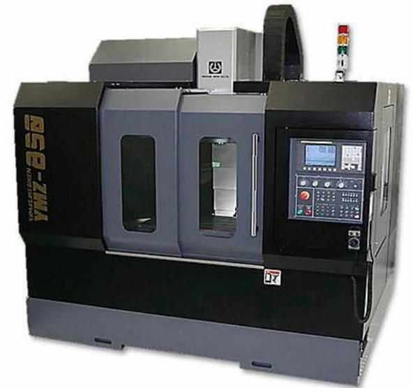
CNC_YMZ850 → YAMAZAKI = 4 MACHINE 800 X 500 X 450
